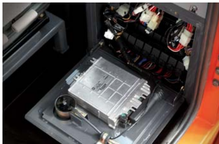
Transmission diagnostics The transmission and engine can be diagnosed using a laptop computer to interface with the diagnostic system.
