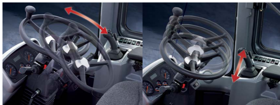
The steering Column The steering column features both tilting and telescopic functions.
