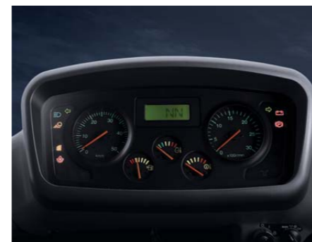
Central Monitor Panel The compact central monitor panel is ergonomically designed and allows the operator to monitor the status and warning lights at a single glance.
