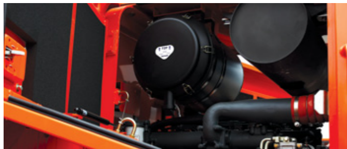
Air-Cleaner Filter The high capacity air cleaner eliminates harmful particles from the air and extends the life of the engine and replacement intervals.
