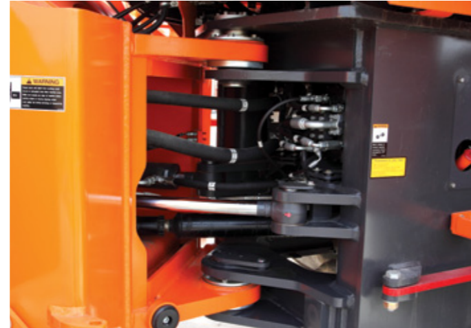
Central Joints A good accessibility at the articulation joint is essential for an easy maintenance.
