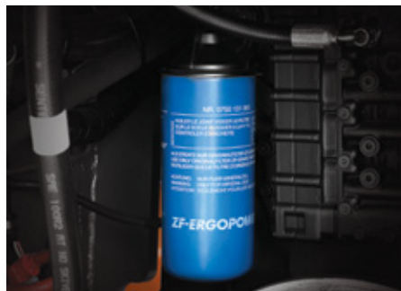
Transmission Filter The transmission filters are within easy reach and like the rest of the machine's service components, can be checked from ground level.
