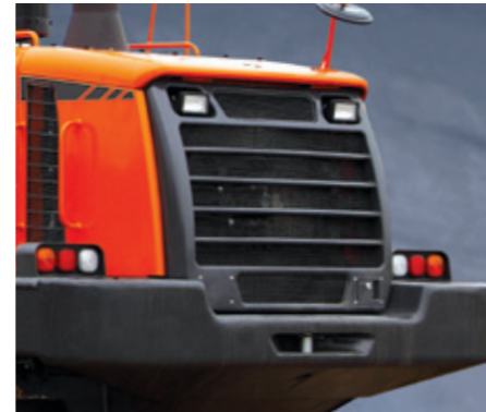
Radiator Grill (Steel structure)
