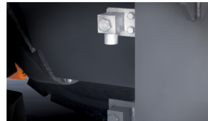
Remote Engine oil & Coolant Drain Remote drain valves have been installed in an easily accessible location for convenient draining of fluids. (Coolant - upper, Engine oil - lower)
