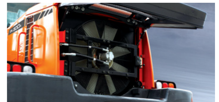
Hydraulically Operated Fan Hydraulically operated fan can swing out and is very easy to clean the cooler cores. Air conditioning condenser is combined with radiator assembly and can be tilt for easier cleaning.
