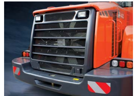
Radiator Grill (Steel structure)
