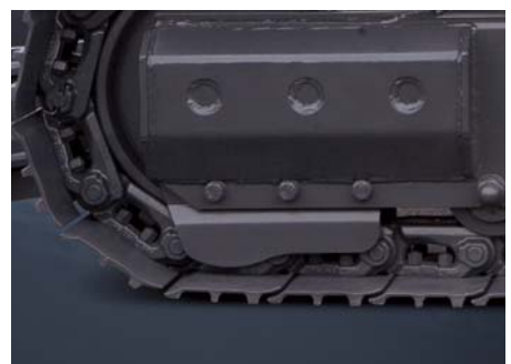
Prefabricated Track Guard The track guard, which protects the vital track components is a prefabricated component and allows for easy replacement.
