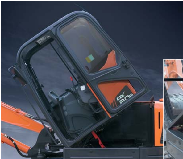
Tilting cabin for easy maintenance
