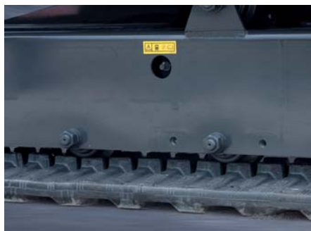
Lower track roller As casting product is replaced by forging product, strength is increased by 75% compared to the existing model, thereby improving wearproof property.
