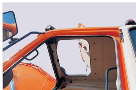
Large ceiling cover The ceiling cover can be opened to confirm the bucket operation even at the maximum excavating height. (Visual range increased by 25% compared to previous machine.)
