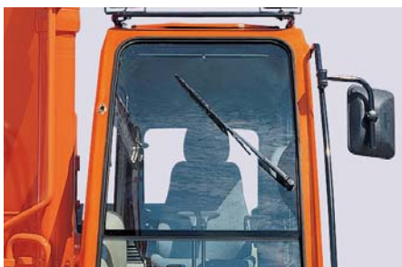
Long wind shield wiper blade Front visibility is further improved by using the lengthened wiper blade (wiper area increased 35% compared to previous machine.)
