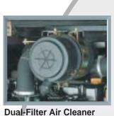
The high-performance dualfilter air cleaner eliminates dust from entering the engine. The cover is a one-touch open/close type allowing easy
