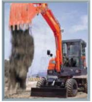
**Powerful Digging Force** Powerful digging force of 4,060kgf(ISO) from the 54.1HP (SAE J1349,net) engine achieves excellent performance quickly within a short time under any working conditions. In addition, a engine control lever is installed on the left control stand in the cabin to make it easy to control working speed.
