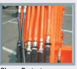
**Sleeve Protector** Sleeve protector with high resistance to wear is equipped to prevent the highpressure hose from being damaged or broken and working oil from splashing when it is damaged.
