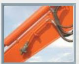
Two Way Piping Line Installed
