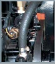
Fan Belt Easy Tension Adjustment and Replacement The spacious area around the fan belt enables easy tension adjustment and replacement. The mounted B-type belt has a greatly extended replacement interval.
