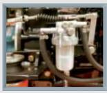
Water separator The transparent glass water separator is mounted at a location easily accessible from the ground allowing easy maintenance of the fuel system.
