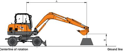
A : Load radius from centerline of rotation B : Load point height Boom : 3.0 m (9'10") Arm : 1.6 m (5'3") Bucket: PCSA 0.173m<sup>3</sup> (CECE 0.15m<sup>3</sup>)
