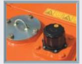
**Air Breather** We designed the hydraulic system for prevent the pump from cavitaion.
