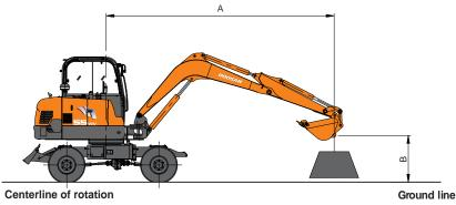
A : Load radius from centerline of rotation B : Load point height Boom : 3.0 m (9'10") Arm : 1.6 m (5'3") Bucket: PCSA 0.173m<sup>3</sup> (CECE 0.15m<sup>3</sup>)
